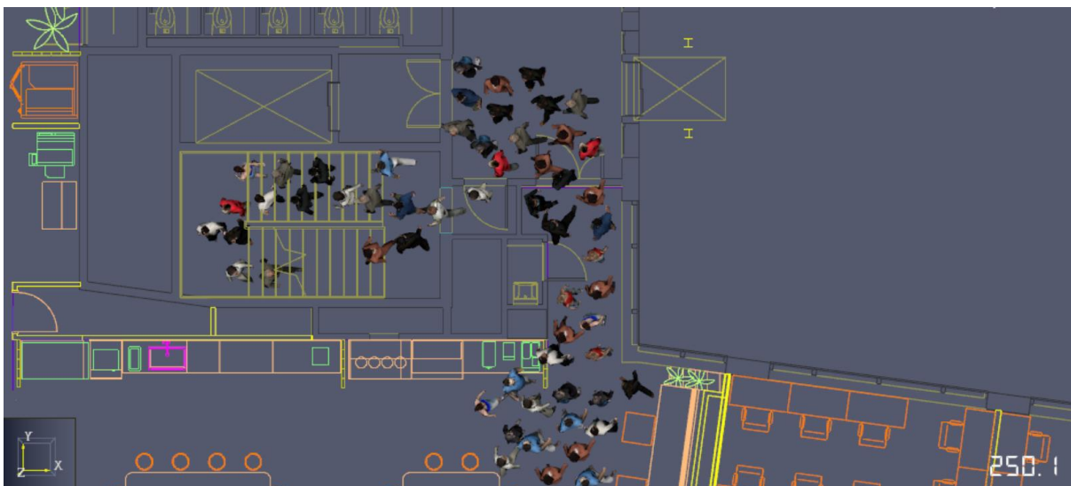
Figure 5: View of the Pathfinder simulation with [speed, size]=[1 m/s, 0.6 m] at t=250 s, floor 6, staircase A
