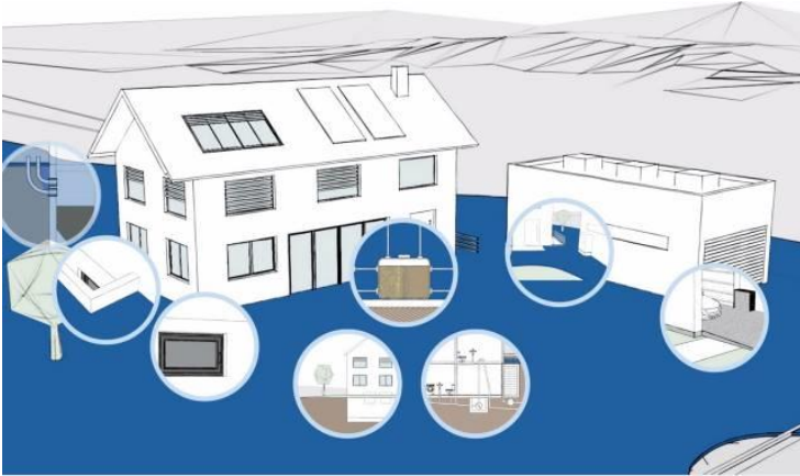
Figure 13: Typical water penetration paths during flooding (origin of the photo: EPZ)
