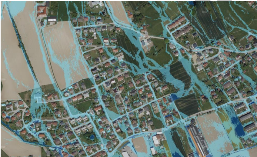
Figure 12: Example of a Heavy rainfall hazard map with the computational simulation of stormwater runoff (the origin of the photo: EPZ)
