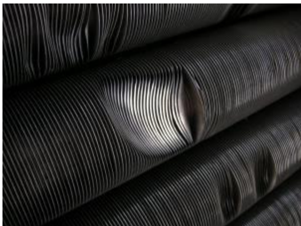
Figure 7 Aluminium lamellas of an air condenser system damaged by hail: detailed view (source: GDV)
