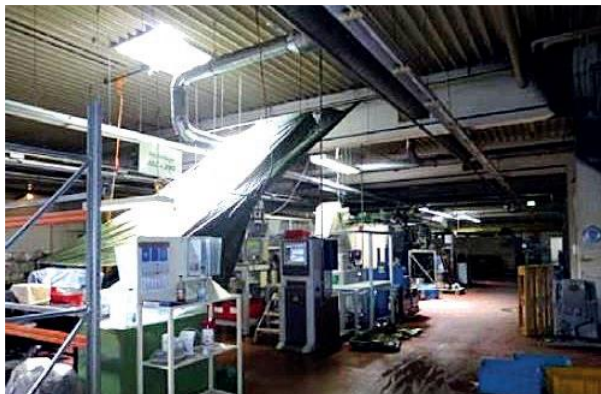
Figure 14 Examples of machine and apparatus protected against rainwater by film (source: GDV)
