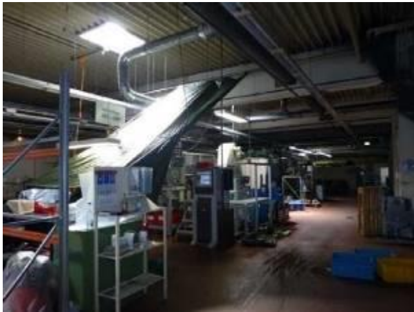
Figure 14 Examples of machine and apparatus protected against rainwater by film (source: GDV)
