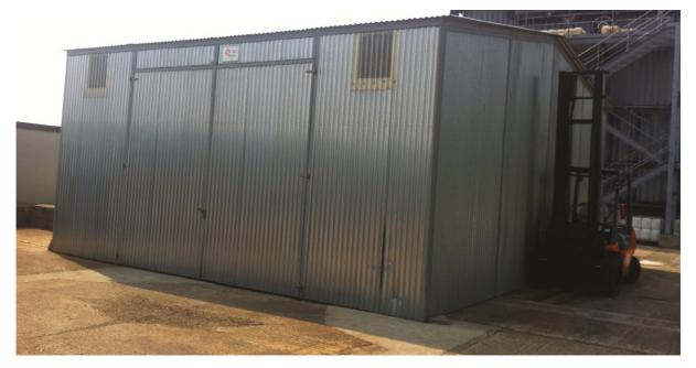
The IMO test facility was used to great effect when the FPA tested fire protected cables for Carnival. The building and its internal clutter was perfect to recreate a representative environment in which the cables were used, and a large liquid fuel spray burner accurately recreated the potential fire threat within a ship's machinery space.
