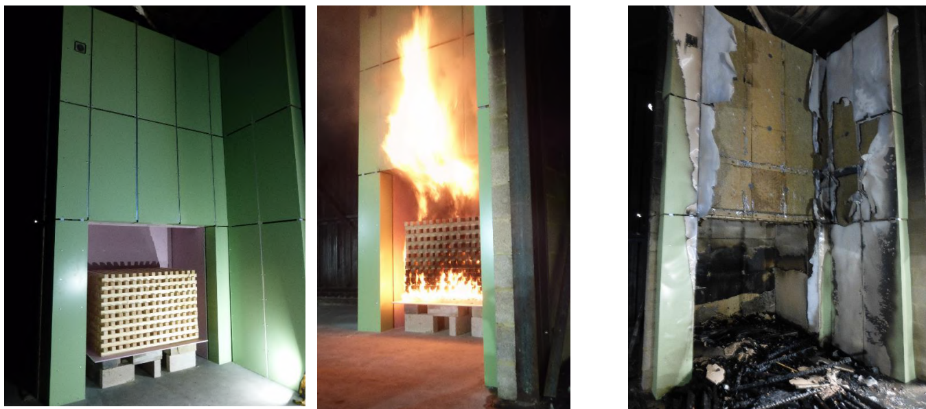
Figure 3 - Stone wool insulated system with A2 ACM panels
