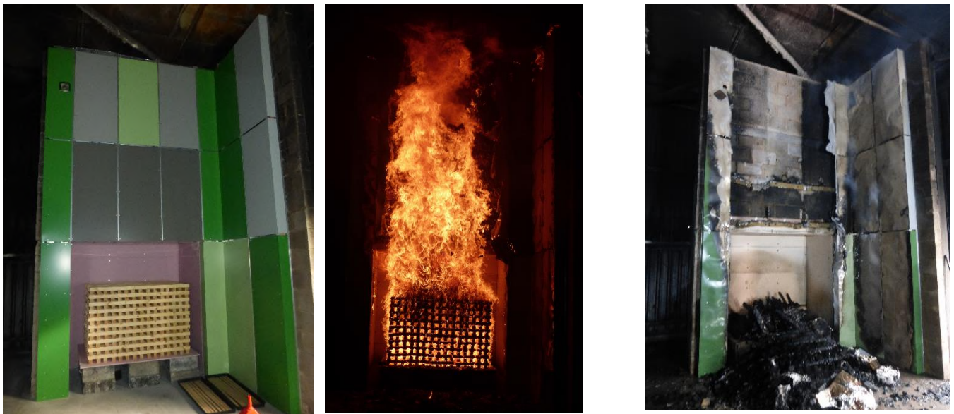
Figure 5 - Phenolic insulated system with A2 ACM panels
