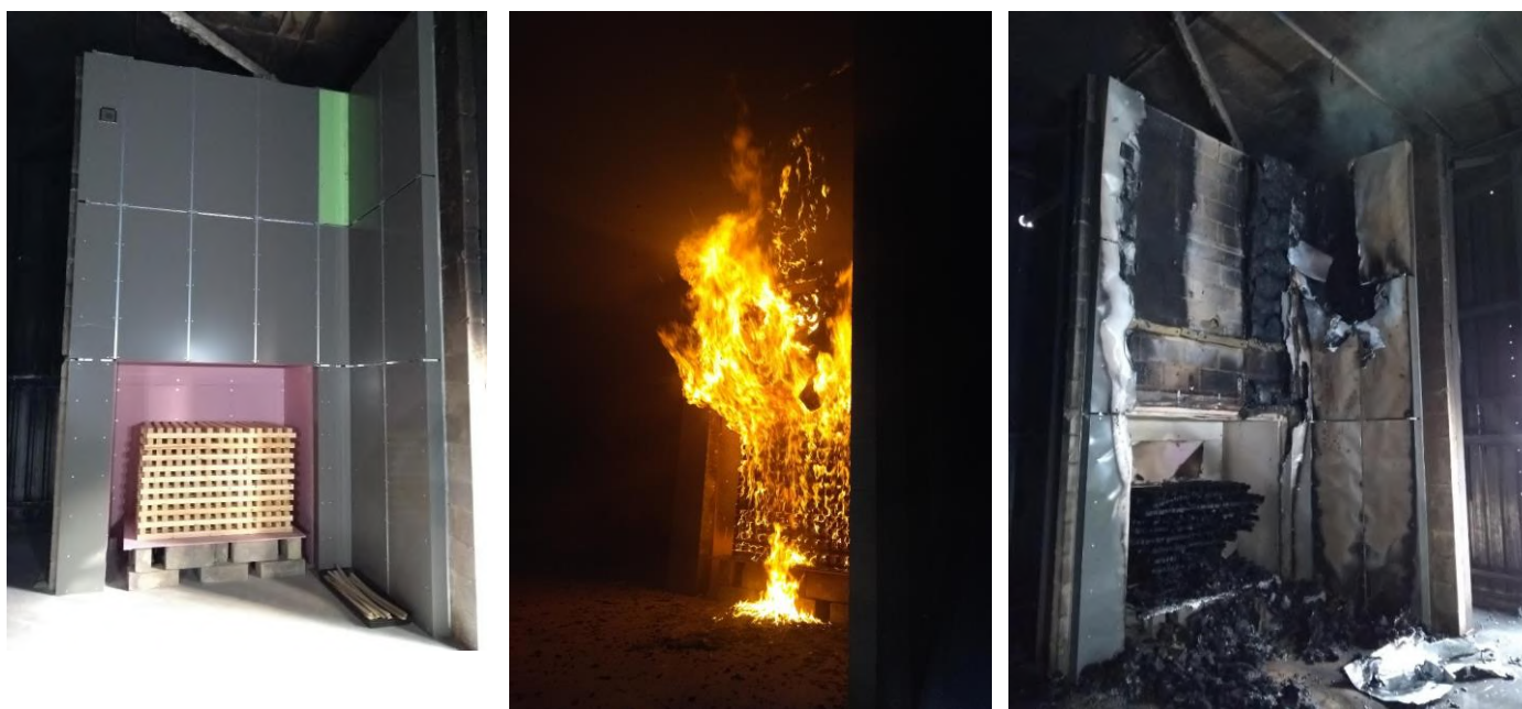
Figure 4 - PIR insulated system with A2 ACM panels
