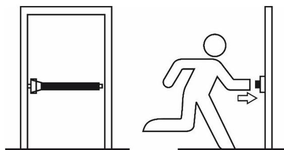
Figure 2 EN 1125 device with touch-bar operation
