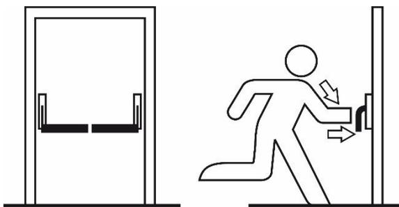
Figure 1 EN 1125 device with push-bar operation
