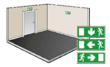
Temporary buildings shall be provided with photoluminescent signs and also with illuminated/luminous signs in those cases where the buildings do not receive daylight. Where illuminated/luminous guidance signs are required, these shall be provided with emergency power that secures the intended illumination for at least 60 minutes.
