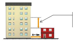
If A is less than 5 m, the facade over a distance of 5 m above the roof of the temporary building must be protected to prevent the spread of fire.
