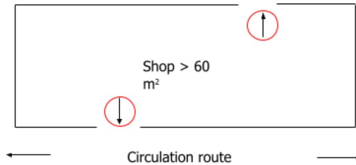
Figure 11: Large shop > 30 persons (ca 60 m 2 net customer area or larger) with requirement for escape facilities at the rear in indoor shopping centre for more than 150 persons
