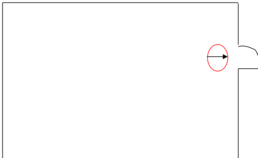
Fig. 18. Small garage with only one escape route, i.e. a travel route no longer than 30 m to doors leading to the open.
