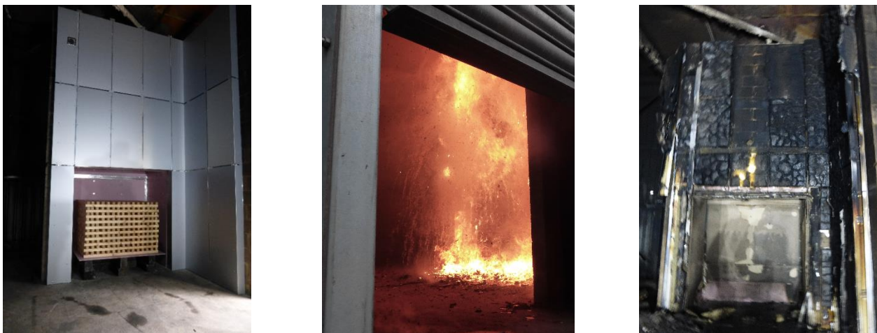
Figure 6 - PIR insulated system with PE ACM panels (note test had to be stopped early, after 12 minutes)
