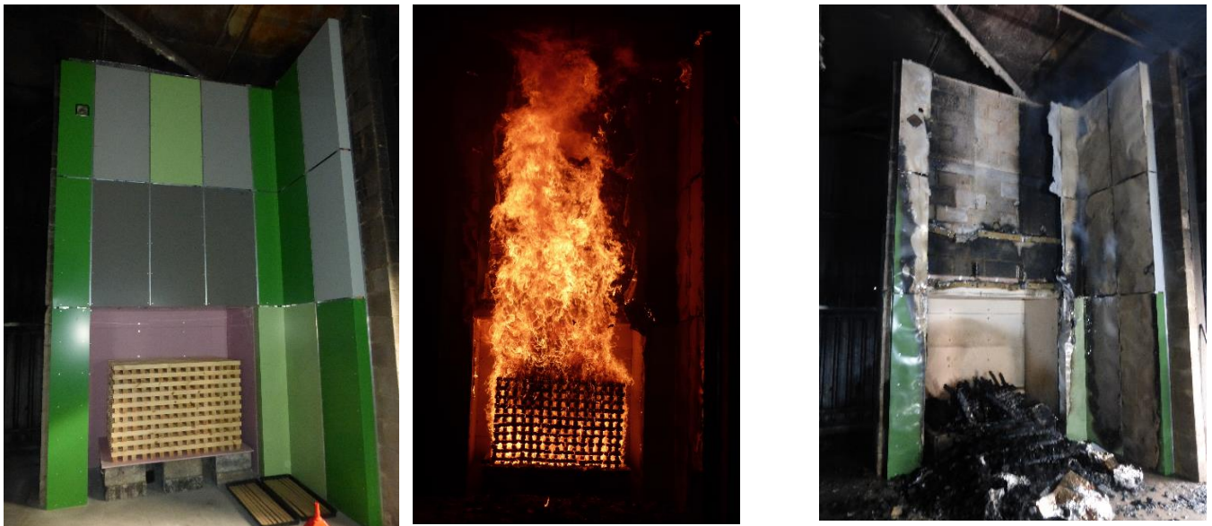
Figure 5 - Phenolic insulated system with A2 ACM panels
