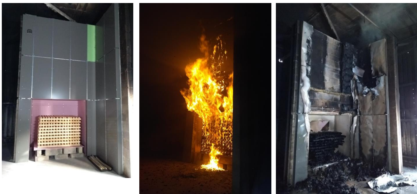
Figure 4 - PIR insulated system with A2 ACM panels
